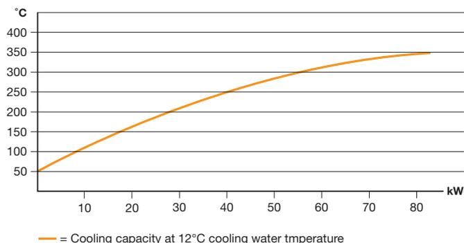
— = Cooling capacity at 12°C cooling water temperature
